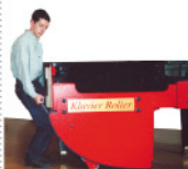
The pivoting leg is used to lift the piano so as to remove the left leg
